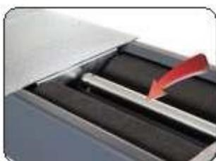
The roller units are fitted with sensors detecting the presence of a wheel set on the rollers. This system prevents the rollers from starting accidentally. The motor automatically stops in case of tyre slipping, thus preventing damage to the tyres.
